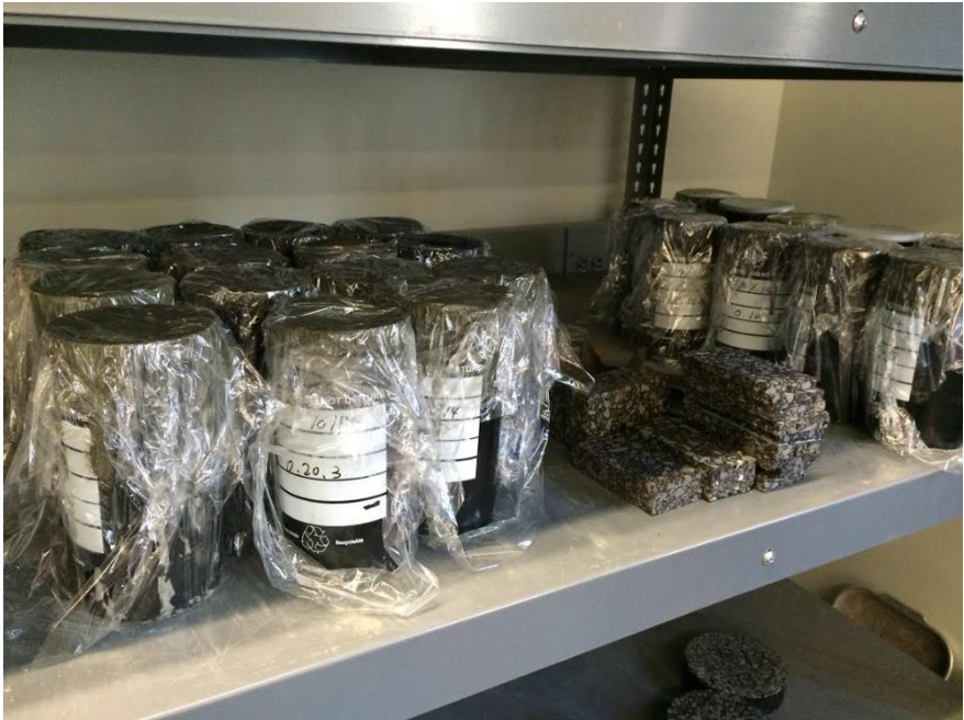
Fig B2: Demolding and Sample Labeling
