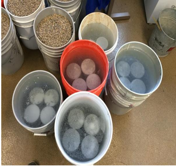
Figure 3. 5: Specimen placed in water for curing days
