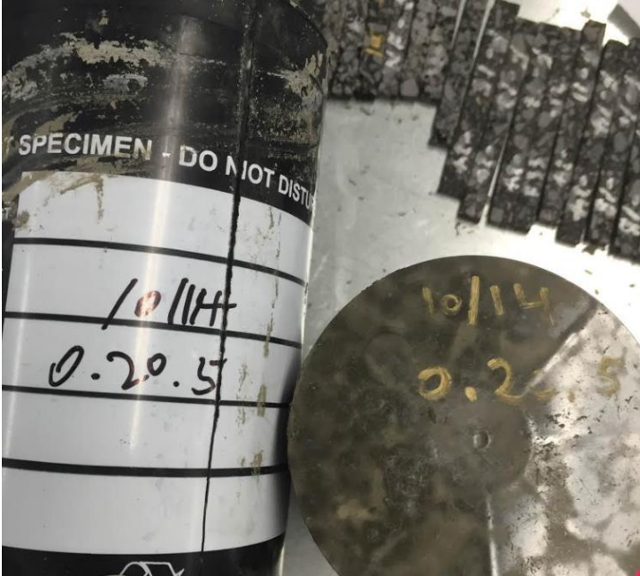
Fig B1: Specimen Storage before Demolding
