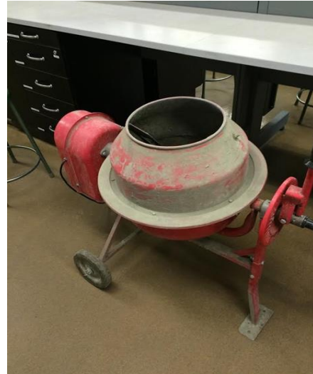
Figure 3. 4: 1.25 Cubic Foot Concrete mixer
