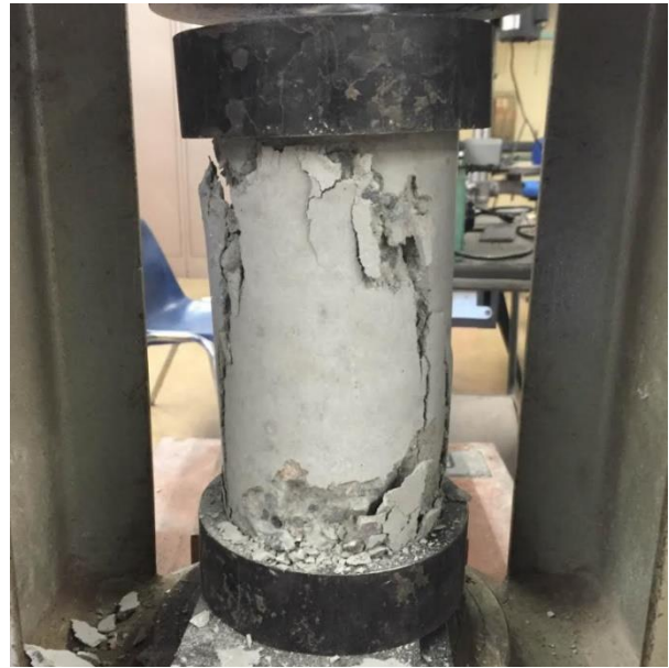
Figure 3. 8. Broken Concrete Sample
